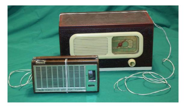
Almost any set with an internal loop, working or not, can serve a a useful DX antenna. The 2-3 turn pickup coil should be wound in the same plane as the windings on the internal. That will generally be around the long dimension on radios with air-core loops, and around the shout dimension for set with ferrite rods.
