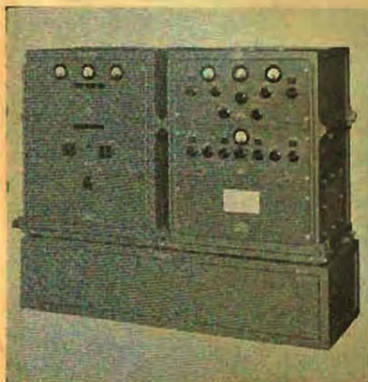
S.T.C. type A.T.20-500 watt transportable radio transmitter designed and manufactured for the R.A.A.F. Production of these equipments which were supplied in large numbers was one of the Company's outstanding achievements.
