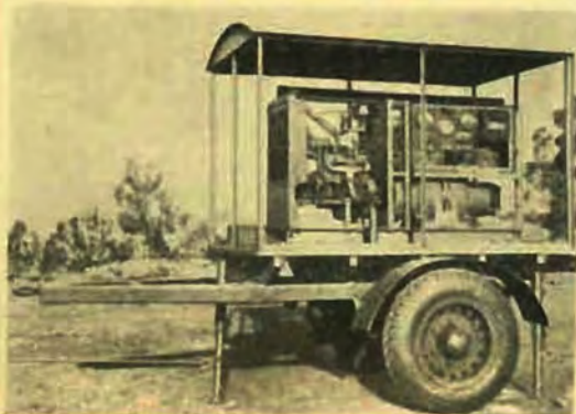
In forward areas, the Services were dependent upon auxiliary power supply sources such as the trailer-mounted Westinghouse-Rosebery 5 KVA generating set shown below.
