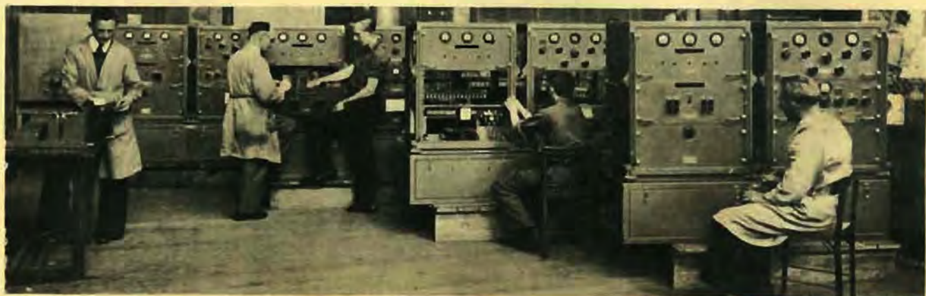
RAAF AT20 transmitters on the production line at the South Melbourne factory of Eclipse.
