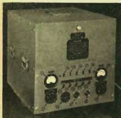
The unit shown above is A.C. power supply unit, type SRA-34, produced by Transmission Products, of Sydney, for the US Forces. This equipment was fully "tropicalised" and provided all operating voltages for a medium-power radio transmitter.
