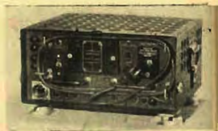
Airzone (1931) Ltd. manufactured the power supply unit shown above to permit AC operation of the SCR-522 by the US Sig. Corps and RAAF. The US identification was AMS-195, while RAAF called it PSU type "V."
