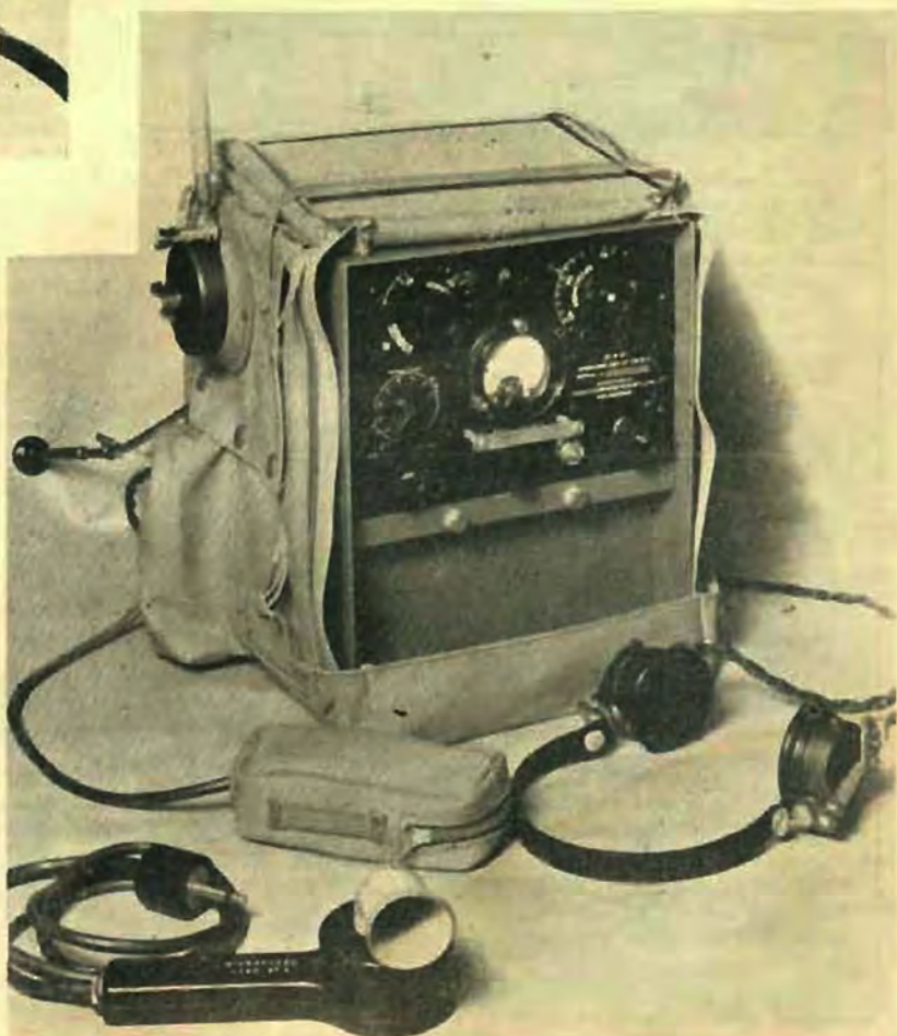
Developed for jungle warfare as a result of experience with the 108 Mk II and the 208, the Army 108 Mk III shown below was built by Radio Corporation and saw extensive service throughout the SWPA. This equipment, like the others on this page, was completely battery-operated and designed for "man-pack" operation.
