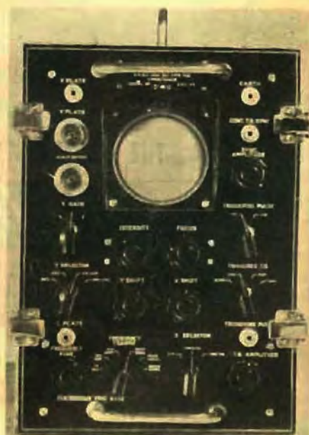
Airzone produced the 5-inch CRO shown at right as part of the radar production programme.
