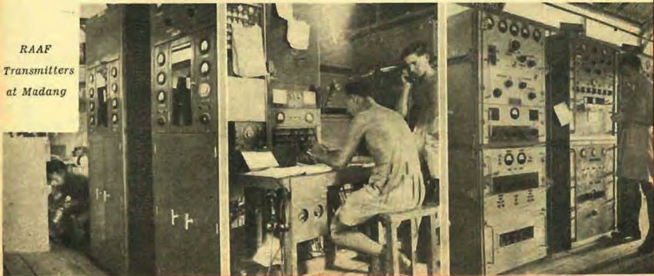
The photograph above and those below show various equipments at the RAAF Telecom Unit transmitting station at Madang. Above are three AT5 transmitters, made by AWA, with line relays for each mounted on the floor beneath each transmitter. Below, from left to right, are: 1. Two AT14S HF transmitters (made by AWA). At the left of the picture one of the station personnel is removing an STC transmitting valve from its packing case. 2. The 50 line patch panel through which all lines feeding into the transmitters are controlled; and 3. An AT17 VHF transmitter, made by Thom & Smith (left) and an AT20 (STC).
