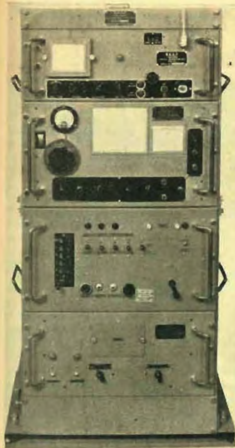
The RAAF type A.12-S assembly shown above is a precision unit developed by Radio Corporation for VHF D/F service. This equipment uses a special crystal calibrator assembly and makes use of the AR17 FM/AM receiver. This equipment was also known as the RC73D.
