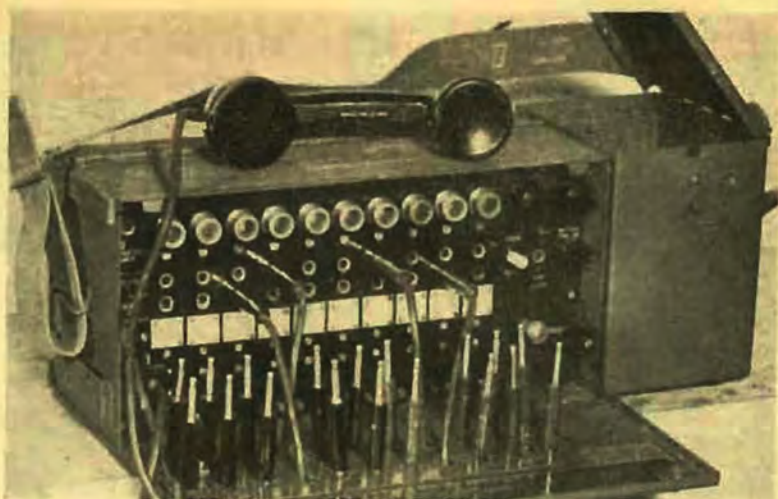
The 10-line telephone switchboard illustrated above was Army's standard equipment during most of the war years. Known as the "U-C" (universal call) board, the lamp indicators of this assembly were extremely sensitive and could be used with buzzer or magneto-call telephones. Standard Telephones were responsible for production of this equipment.
