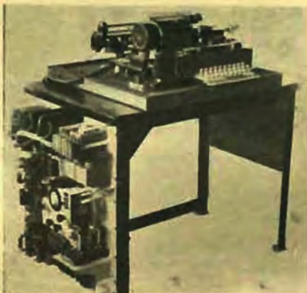
The "Telex" unit shown above, with its covers removed, is typical of a quantity produced by PMG Workshops for the RAAF to permit teleprinter operation over normal line circuits.
