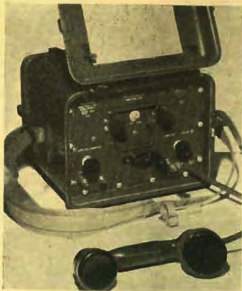
The assembly shown above is a tropicalised high-power telephone produced by Kriessler Radio for the Army. In addition to a magneto-call telephone, the equipment included an amplifier to permit efficient operation over long distances.
