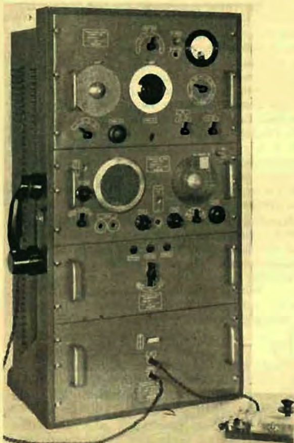
Philips Electrical Industries produced the "DR101" transmitter-receiver illustrated at left for the US Navy. Capable of operation from AC or battery supply, this assembly had a power output of 40 watts and operated in the 1.8 to 3.1 MC/s range.
