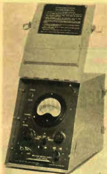
Designed primarily for radar maintenance work, the battery-operated electronic megohmmeter illustrated above was produced by HMV. An AC-operated version also was produced.
