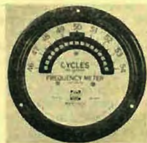
Reed-type panel mounting frequency meters were a critical item until A. J. William commenced Australian production. One of the firm's "SR6" series of frequency meters is illustrated.
