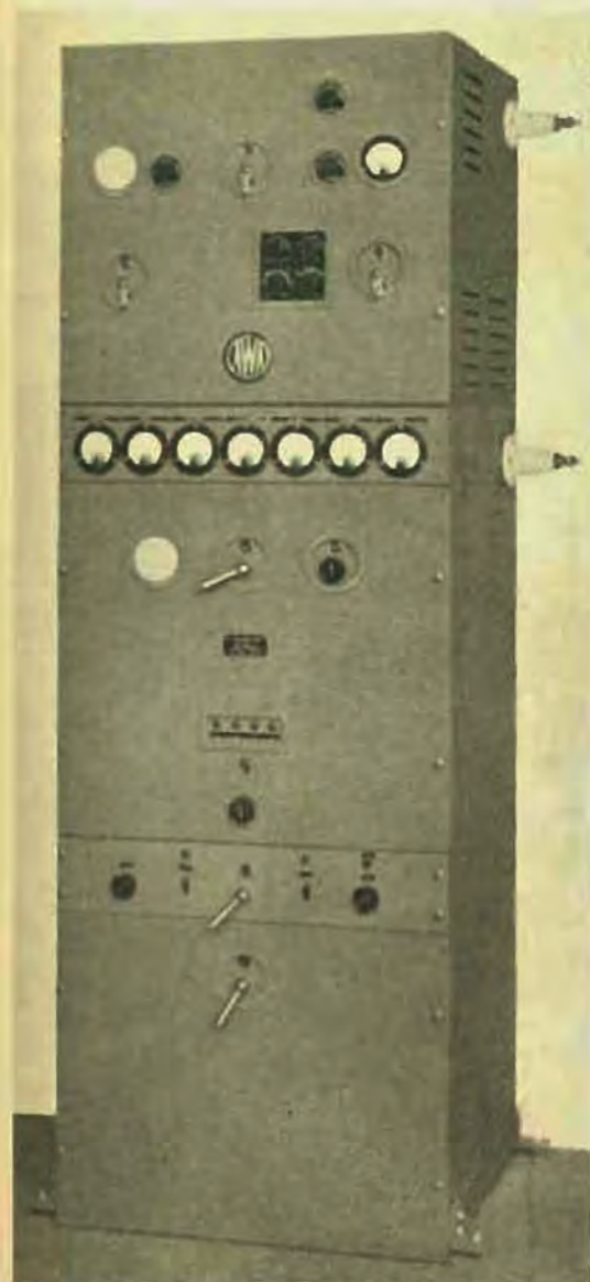
The RAAF transmitter illustrated above operates on 100-150 MC/s., and provides frequency- or amplitude-modulated VOC transmission with a power output of 50-150 watts. Known as the "AT17," this mobile or static equipment was manufactured for the Air Force by Thom & Smith Pty. Ltd.
