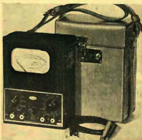
Radio Equipment, of Sydney, made the versatile multimeter shown above. Known as the "D8," this instrument was specially designed for Service use.
