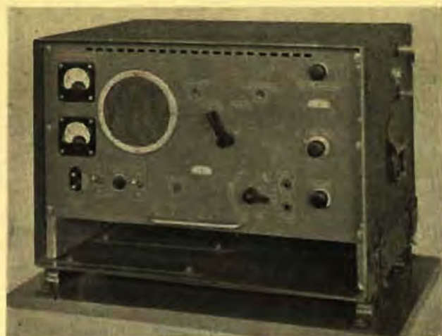
The compact transceiver illustrated above was produced by Philips Electrical Industries for the RN, RAN and USN. Known as the "DR106," this equipment is a 20-watt assembly working in the 60-80 MC/s. range and can be operated from battery or AC power supplies.
