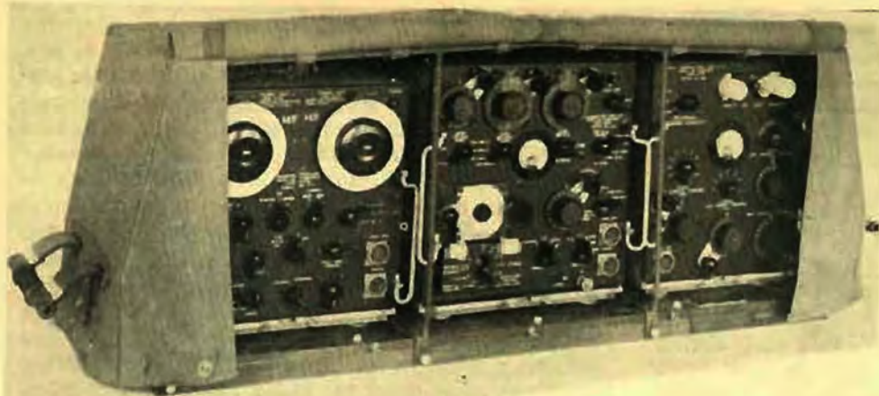
Illustrated at left is the justly-famous "AT5/AR8" which was made to RAAF specifications by Amalgamated Wireless. This general-purpose aircraft equipment comprised a 50-watt transmitter operating on medium and high frequencies and a receiver, and in addition to providing crew intercom, could also be used for D/F and homing. Army used a slightly modified version as WS No. 112.
