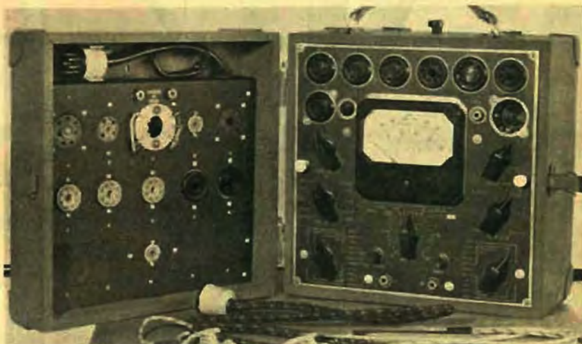
Illustrated above is Transmission Products' type "VCT-V" valve and multi-tester assembly which was produced for Service Workshops.
