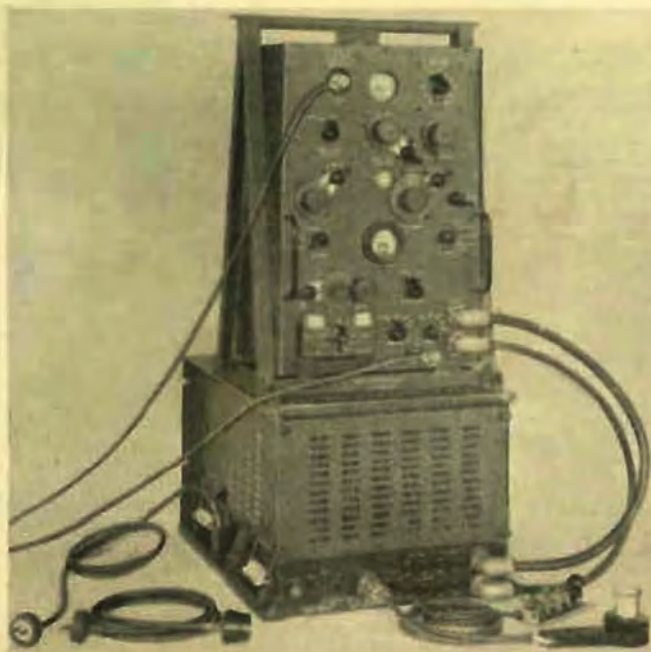
Known variously as the "TW-12" and the "AMT150," the compact assembly shown below was developed by A.W.A. for the U.S. Forces and provided 15-50 watts output on RT, MCW or CW in the range from 1.5 to 16 MC/s., with provision for 6 "spot" frequencies. A similar assembly, rated at 80W., was produced for RAAF as the "AT21."
