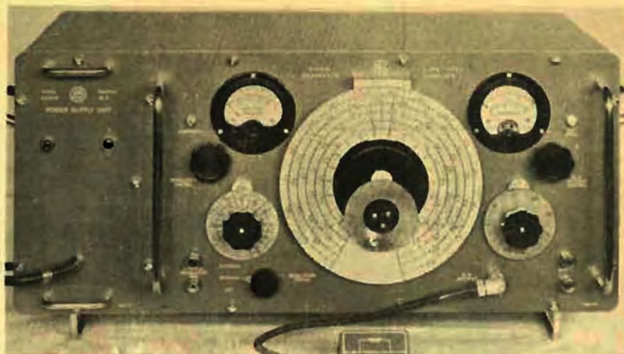
The elaborate signal-generator illustrated above is the R7231 produced by Amalgamated Wireless for use in Service and production design laboratories. Built to a high degree of precision, this instrument provides coverage from 95 KC/s. to 30 MC/s. in ten bands.
