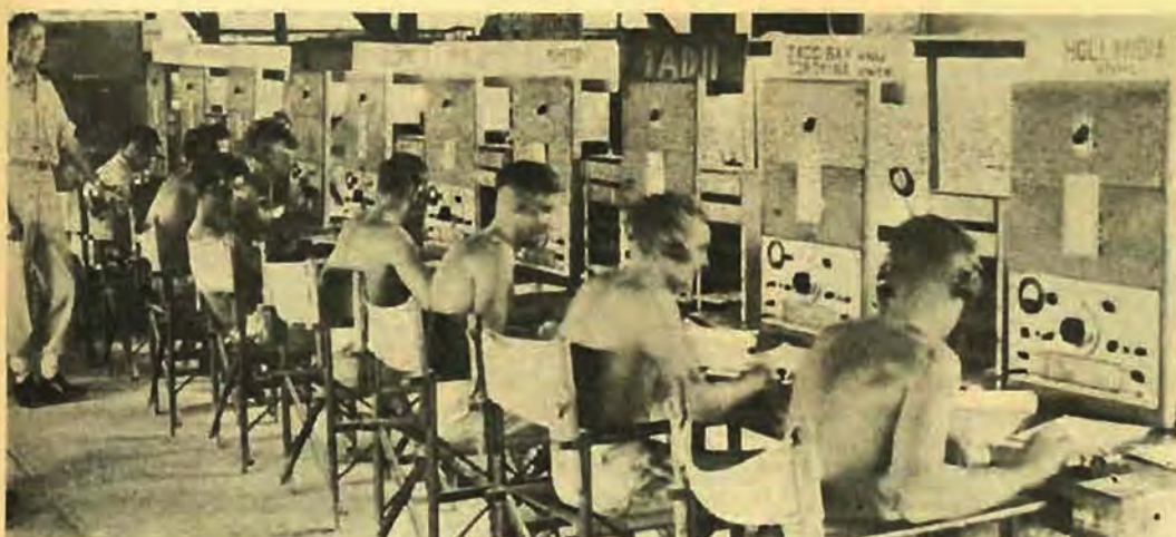
★ A bank of AR7 receivers, made by Kingsley Radio, at the Telecom Unit receiving station at Madang can be seen at left. Call-signs and locations of some of the stations being worked can be identified on the picture. There were about 27 of these receivers in use in this signals office. ★
