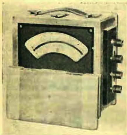
A. J. William, of Melbourne, produced some fine examples of sub-standard instruments and one of the firm's 5 1/2 in. scale type P16 portable instruments is shown at left.
