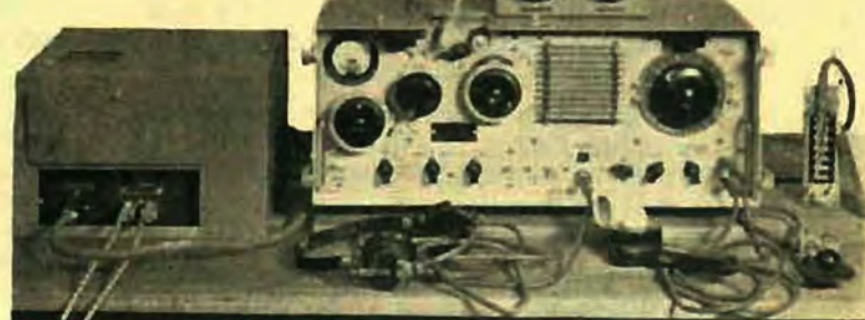
The versatile transmitter-receiver shown above was developed by Radio Corporation for the RAN and was known as the "RC8." This equipment had a power output of over 10 watts and operated in the 3-10 MC/s range. Major application of the RC8 was in the Navy's "small craft," where it did a particularly fine job.
