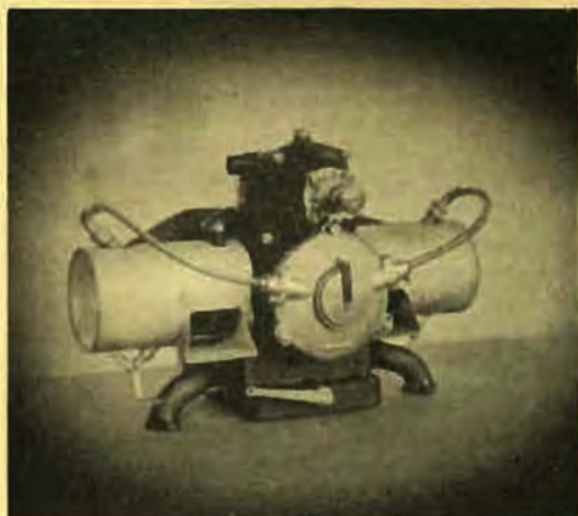
The "Enfield" twin-cylinder petrol motor shown above was made by K.L. Engines & Tractors, of Melbourne, as the prime mover for a 2.75 KVA alternator set which was widely used for Radar power supply.
