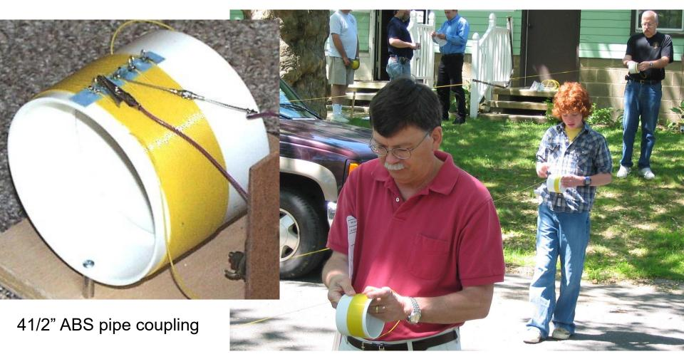
Anchor the end of the wire and maintain tension while winding. Cardboard strip raises the turns to be tapped.
