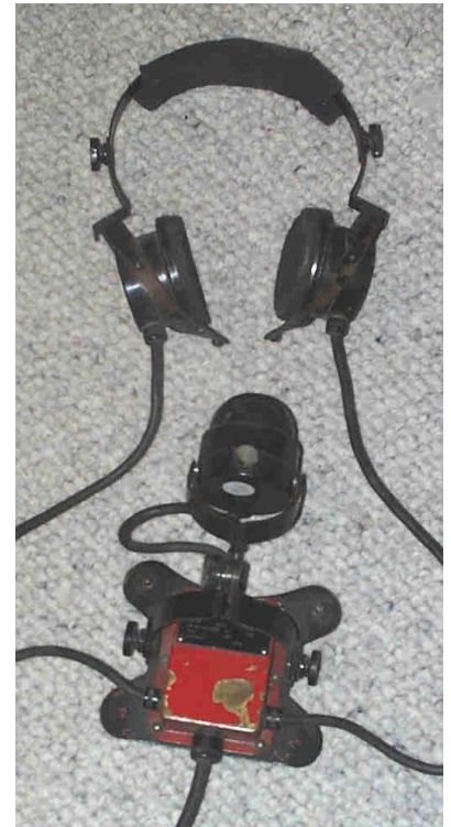
Navy “Deck Talker” Sound-Powered Telephone
