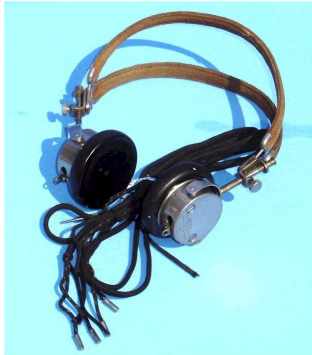
“Head Telephones” Western Electric 509W
