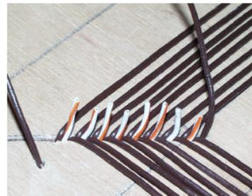
Insert a short scrap of wire in the kerf after every two turns to achieve proper spacing.
