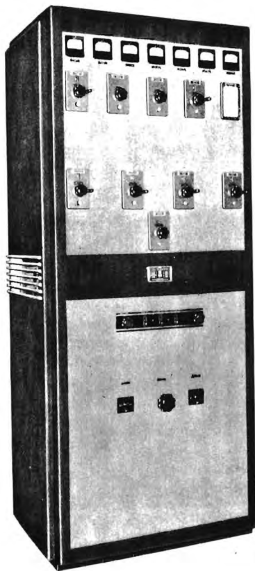
ET-4331 COMMUNICATIONS TRANSMITTER 1 KW, 3 TO 20 mc.
