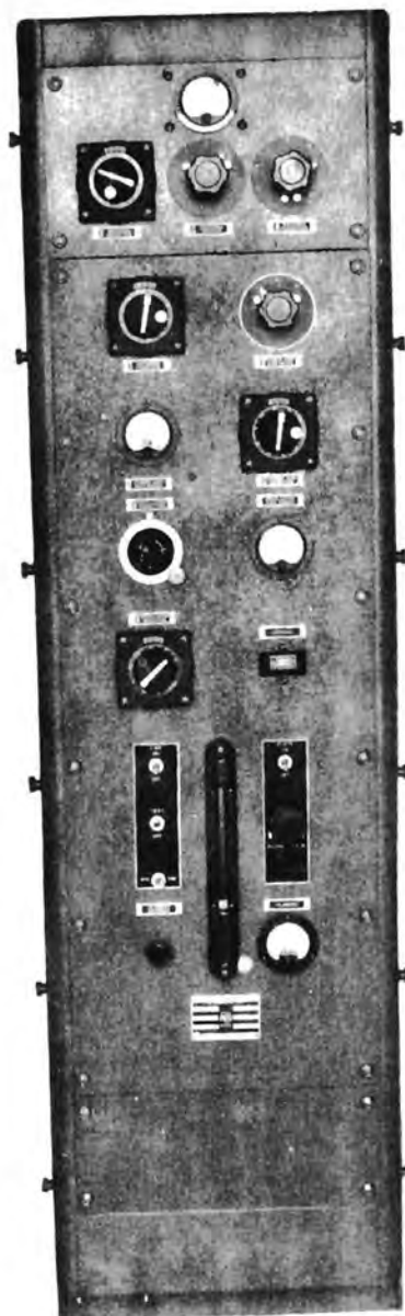
ET-4336 COMMUNICATIONS TRANSMITTER 2 TO 20 MC., 350 WATTS
