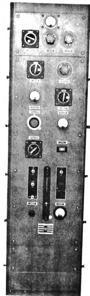
250 WATT GENERAL PURPOSE COMMUNICATION TRANSMITTER. ET4336G.
