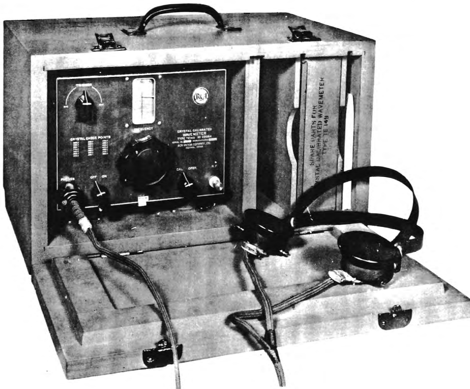
CRYSTAL CALIBRATED FREQUENCY METER EQUIPMENT. TE 149
