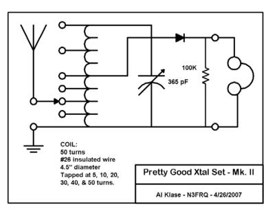
The target value for the cap is 365 pico-farads (mmF or pF), but a 500 pF unit as found in some of the old battery sets will work nearly as well. You could also use the large half of the two-gang cap from a junked all-American-five radio, etc.
