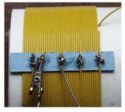
$50^{\text{th}}$  turns on top of the cardboard. Holding the wire firmly in place with your left thumb, clip the wire leaving about a foot to terminate the coil. Drill two more holes in the form just beyond where the  $50^{\text{th}}$  turn crosses the cardboard, and lace the end of the wire through them.
