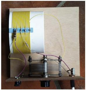
the coil in the approximate orientation shown so it can be coupled to the antenna tuner to be described in "Phase II."
