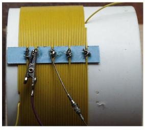
The best option, for maximum performance, is silver-plated Teflon-insulated hook-up wire if you have any in the junk box, but even common vinyl-insulated tinned stranded wire will work all right. Close-wound magnet wire is a bad bet, as eddy currents in the adjacent turns cause considerable loss.
