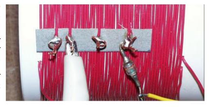
pocket. Lace the end of the wire into one hole and out the other, leaving about a foot protruding from the form. Grasp the coil form firmly and pull the wire taught against the tied off end. Wind 5 turns on the coil keeping the wrie close-wound and tight. Place the end of the cardboard strip under the 5th turn. Wind four more turns, sneaking them under the strip. Wind the 10th turn over the strip. Continue winding placing the  $20^{th}$  and  $30^{th}$
